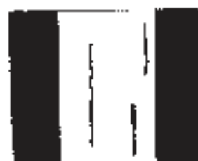
Appearance on the X-ray picture Long, more or less contours parallel with the weld.
